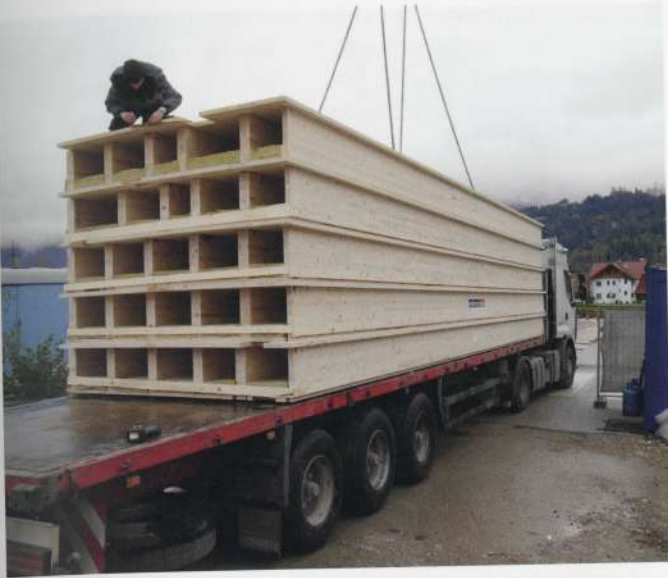
3.1.5 LVL-glulam floor cassettes for Kuchl Campus Extension Building. See case study for more information on project. Source: Dietrich | Untertrifaller Architekten
