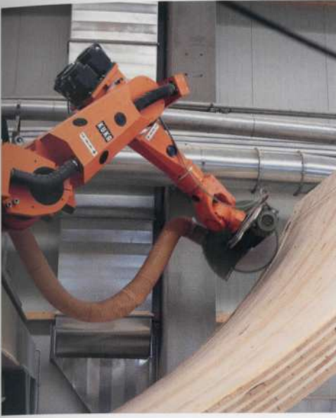
3.1.16 Manufacturing wood components using a robotic arm CNC machine. Source: MERK Timber, Aichach, Germany ( www.merk.de )
